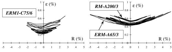
Figure 3. Measured strain ( $\epsilon$ ) in the FRP belts versus drift angle (R).
