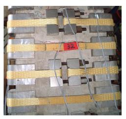
Figure 1. Pre-tensioning technique for carbon (left) and aramid FRP belts (right).
