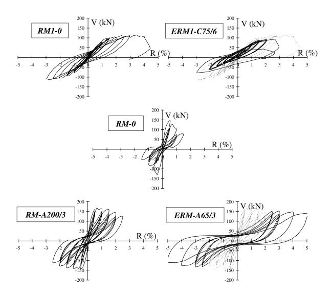
Figure 2. Measured lateral strength (V) versus drift angle (R) for test columns.
